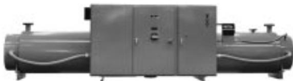
**Fuel Gas Preheater:** This 156 KW fuel gas preheater is used to raise the temperature of fuel gas above the dew point. The design rating is 600 psi at 80° F. The heater has an explosion-resistant terminal enclosure and thermocouple sensor junction boxes.
