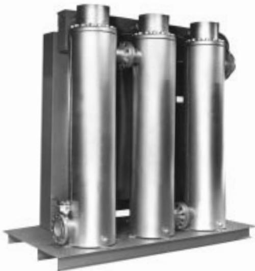
**Fuel Oil Heater System:** A 209 KW fuel oil heater which includes a built-on Vernier control system. The low watt density requirements resulted in a 20 foot long vessel design with immersion heaters inserted at each end.
