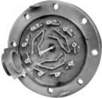
**Large Diameter Elements** - Elements measure .475" O.D., providing extra electrical insulation for superior dielectric strength. As a result, elements are suitable for line voltages up to 600 volts. At the same time, uniform heat transfer from coil to sheath is assured by compacting the insulation in high pressure rollers, then repressing all bends to insure insulation integrity in this critical area. Copper sheathed elements are silver soldered to the flange; all other materials are welded.
