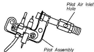
Figure 27 - Pilot Inlet Air Hole
