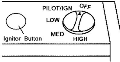
Figure 17 - Control Knob in The OFF Position
