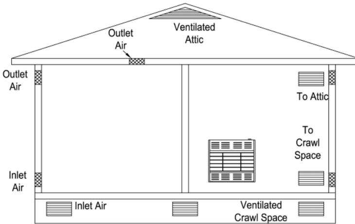
Figure 3 - Ventilation Air from Outdoors
