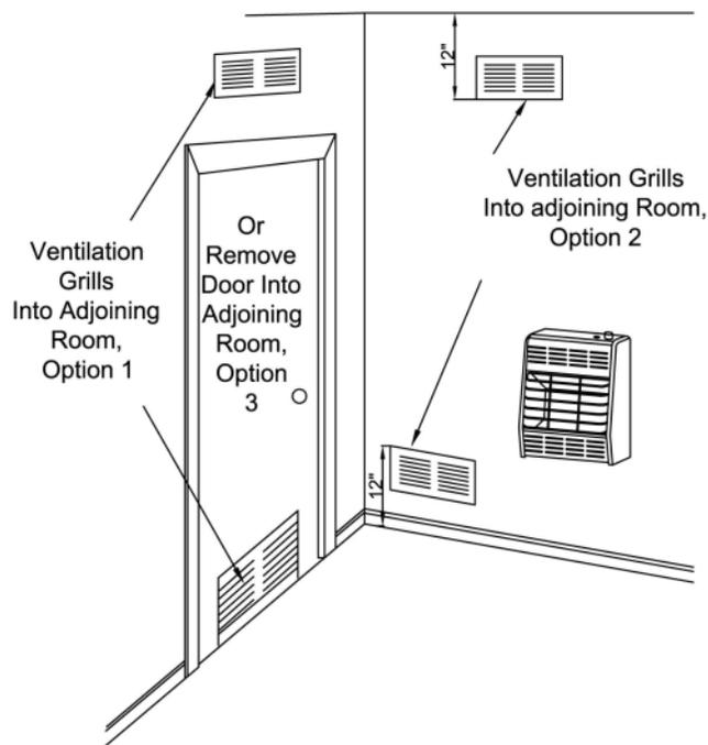
**WARNING:** Rework worksheet, adding the space of the adjoining unconfined space. The combined spaces must have enough fresh air to supply all appliances in both spaces.
