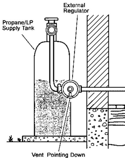
**Figure 13 - External Regulator with Vent Pointing Down**
