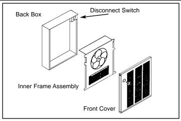
FRAS-1 is 1" deep, allowing the heater to extend into the space 2" while the FRAS-2 is 2" deep allowing for a 3" extension of the heater out of the wall.
