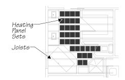
5P. On the drawing, layout the position of the sets of heating panels. Distribute the heating panels evenly throughout the room. Retain this drawing for reference during installation.
