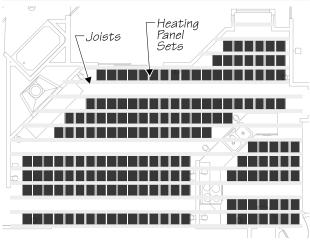
6. Each separate set of heating panels will require 2 connectors and 2 insulators.
