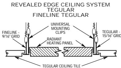
Tegular and Fine line Tegular panels are supplied **standard** with universal mounting clips installed for support chain.
